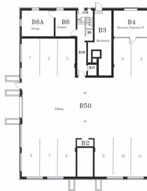
Purin Hall, Existing Ground Floor Plan
